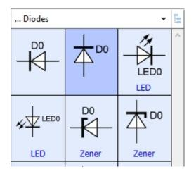
The components are simply dragged from the library onto the drawing **(drag & drop)**. To do this, click with the mouse on the desired component in the library. With the mouse button still held down, drag the component to the desired position on the drawing. There you release the mouse button again.
