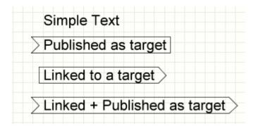
All possible jump targets receive an arrow pointing inwards on the left side. All links with a target are given an arrow pointing outwards on the right-hand side. This identification makes it possible to immediately identify which text elements are linked.
