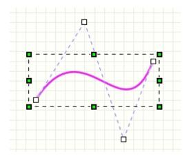
A simple bezier curve always consists of exactly 4 points. You can also define several curves in one go. The end point of the last curve is then automatically used as the starting point of the next curve, so that 3 points (2 control points and 1 end point) are sufficient for each additional curve. bezier curves therefore always consist of at least 4 points and 3 points for each additional curve, i.e. either 4,7,10,13, ... points in total.
