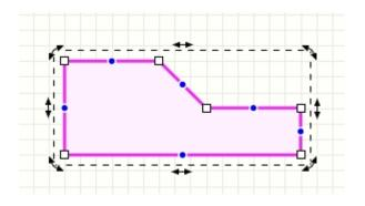
You can also create new additional nodes at a later date. For this, there is a so-called **virtual node** in the middle of each line segment, shown as a blue circle. If you click on it and move it, this virtual node becomes a new real node. So you can interactively expand your line with new nodes.
