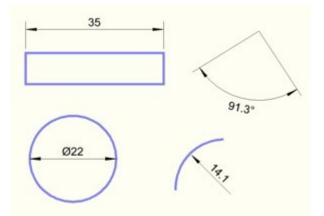
Depending on the type, a dimension consists of 2-3 control points. These control points are set one after the other when creating a new dimension. The control points can then be moved again at any time with the help of the <u>changer</u>.
