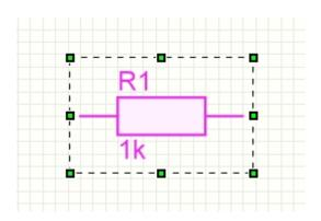
With these sizers you can freely scale the element. If you move the mouse over one of these sizers, you will recognize the possible stretching direction from the changing mouse pointer. Just click on the sizer you want and drag the mouse in the direction you want. The element can be enlarged, reduced, compressed or stretched as required.
