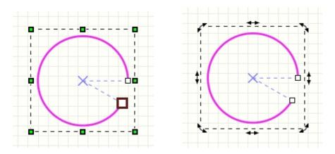
With the <u>changers</u> you can determine the start and stop point of the circular outline. In this way you can create arcs or segments (with filled circles).
