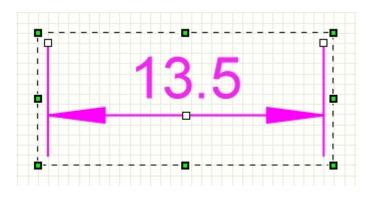
With the <u>changers</u> you can now reposition all nodes of the dimension. So you can easily change the dimensions afterwards.
