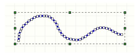
You can also create new additional nodes at a later date. For this, there is a so-called **virtual node** in the middle of each line segment, shown as a blue circle. If you click on it and move it, this virtual node becomes a new real node. So you can interactively expand your line with new nodes.
