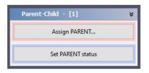
You can also select several components at the same time and set the **parent** for all selected components together. So if you have a contactor and 3 contacts as in the example above, then select the 3 contacts and then assign all 3 components with the contactor as a **parent**.
