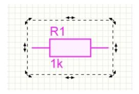
With the arrows you can now **turn** and **shear** the element as you like. Use the 4 semicircular corner arrows to turn. The angle of rotation always locks into the angle of rotation snap you set. You set the rotation angle snap in the lower toolbar:
