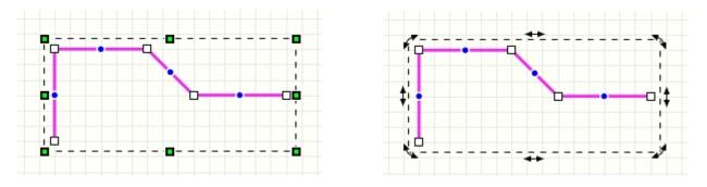
You can also create new additional nodes at a later date. For this, there is a so-called **virtual node** in the middle of each line segment, shown as a blue dot. If you click on it and move it, this virtual node becomes a new real node. So you can interactively expand your line with new nodes.
