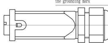
The grounding line connect to the grounding mark
