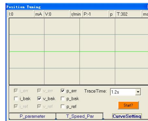
Figure 6-20: Digital Scope settings for the tuning
