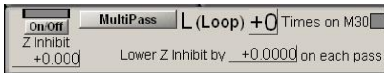
Figure 6.19 – Automatic Z control
