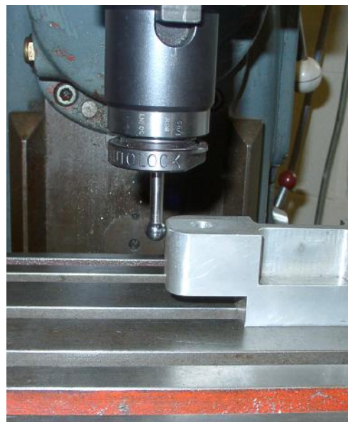
Figure 7.12 - Edge-finder in use on a mill
